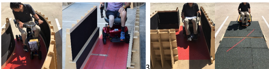
Figure 2: Left to right – Swept Path Test, Narrow Access Path Test, Allocated Space Test, Pavement Gap Test
